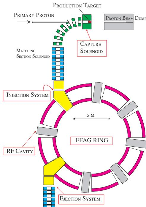
Figure 1: A schematic layout of PRISM
