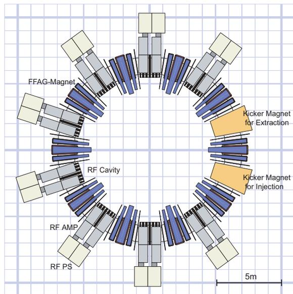
Figure 2: Schematic layout of the PRISM-FFAG
