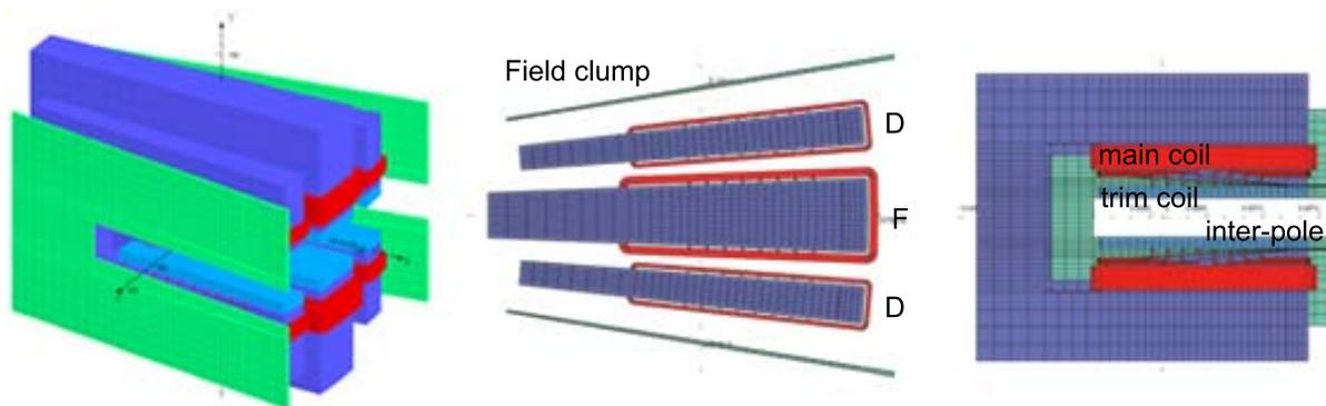
Figure 3: Schematic views of a PRISM-FFAG magnet. A bird's-eye view (left), a top view (center) and a side view (right).
