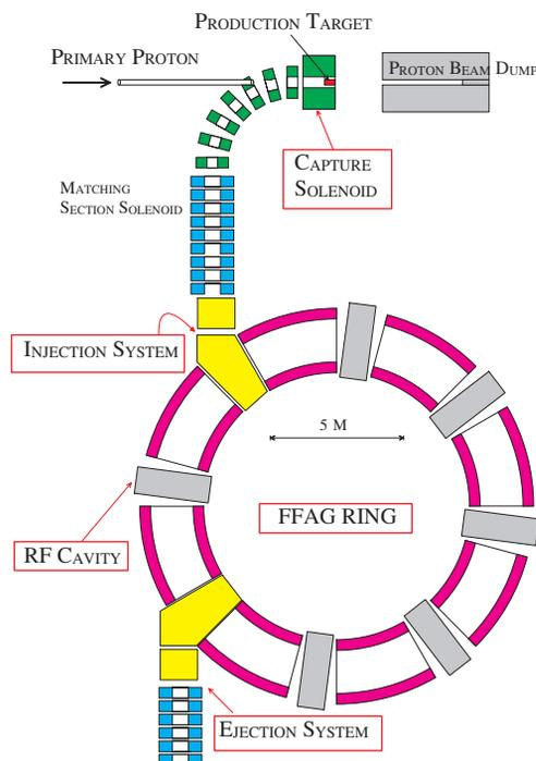
Figure 1: A schematic layout of PRISM
