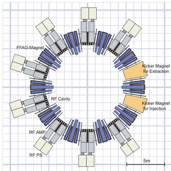
Figure 2: Schematic layout of the PRISM-FFAG
