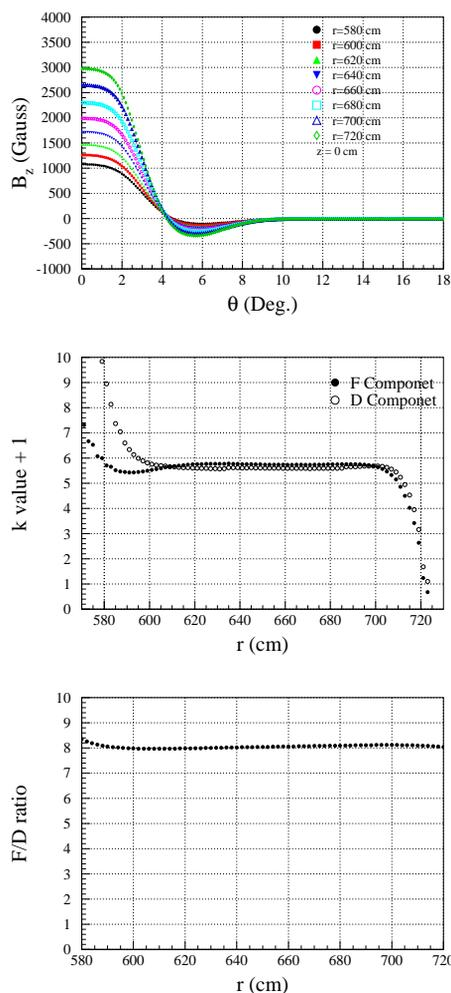
Figure 4: Calculation results of the magnetic field using TOSCA.
