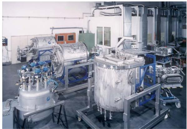
Figure 3: Assembly area of the SRF modules at ACCEL. In the upper right part the clean room class 100 can be seen where the modules need to be assembled in whenever the cavity vacuum is touched.
