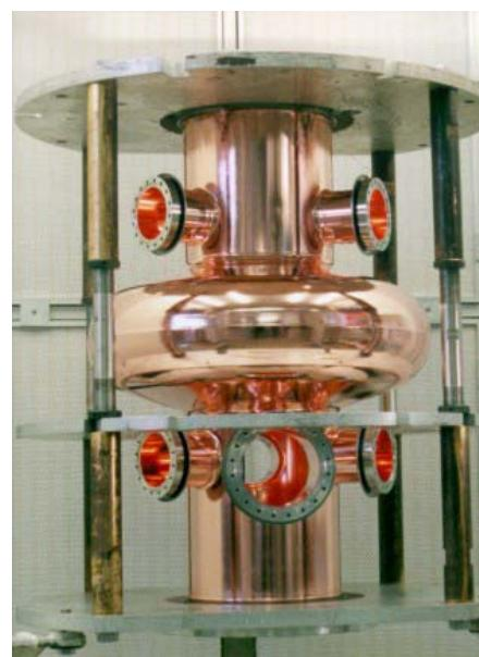
Figure 1: Single cell 400 MHz LHC cavity before sputtering with niobium.
