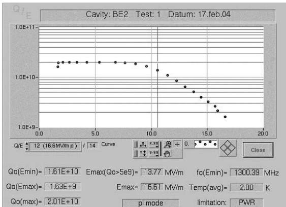
Figure 7: Test result of first prepared TESLA cavity BE1. Field emission was observed above 10 MV/m.
