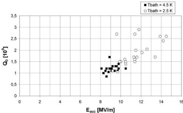
Figure 3: Highest gradients Eₐcc and quality factors Q₀ at the highest gradients achieved at bath temperatures of 4.5 K and 2.5 K in the 21 LHC 400 MHz single cell cavities. The tests were carried out at CERN.
