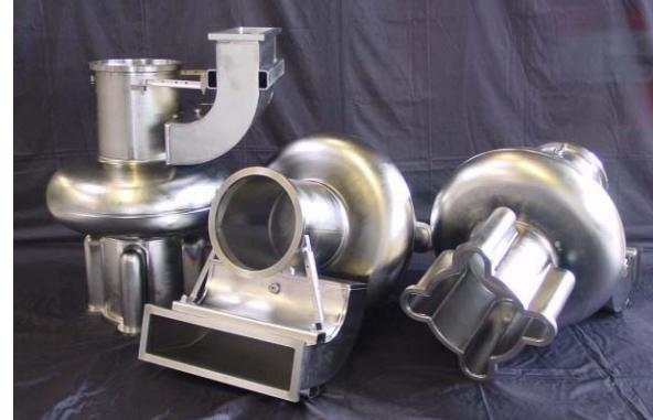
Figure 4: Three 500 MHz cavities of the Cornell design after production and prior preparation.
