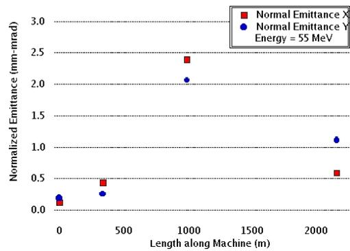
Figure 3: Emittance measurements for the 55MeV injector/dump energy.
