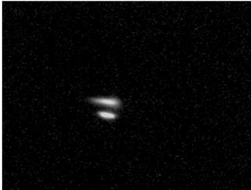
Figure 2: Synchrotron light image in Arc-1, showing the presence of the accelerated and energy recovered beam.
