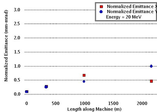
Figure 4: Emittance measurements for the 20MeV injector/dump energy.
