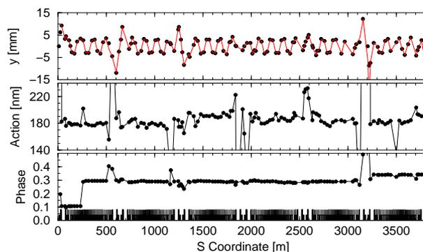
Figure 4: Difference orbit action and phase analysis. In the top graph the measured difference orbit is plotted as filled circles; the curve is the modeled orbit for the average action and phase of each arc. Comparison show excellent agreement between model and measurements.
