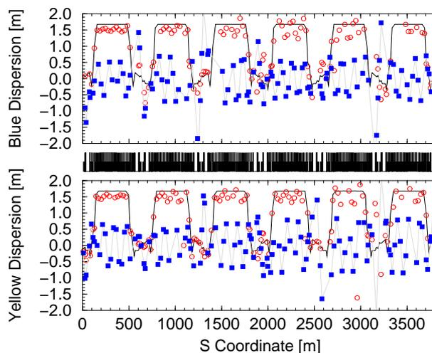
Figure 1: Dispersions measured in low-beta conditions on Nov 1 with gold ions in both RHIC rings. Measured horizontal dispersions are red open circles, and design horizontal dispersions are black lines; vertical dispersions are filled blue boxes. Radial steering was 2 mm. There is clear indication of dispersion coupling from low-beta triplets.
