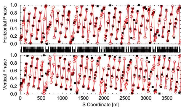
Figure 3: Measured (solid square) and design (open circles) betatron phases in the RHIC Blue ring, Jan 7 16:53, ramp 2163, using beam oscillations for 50 turns after injection.
