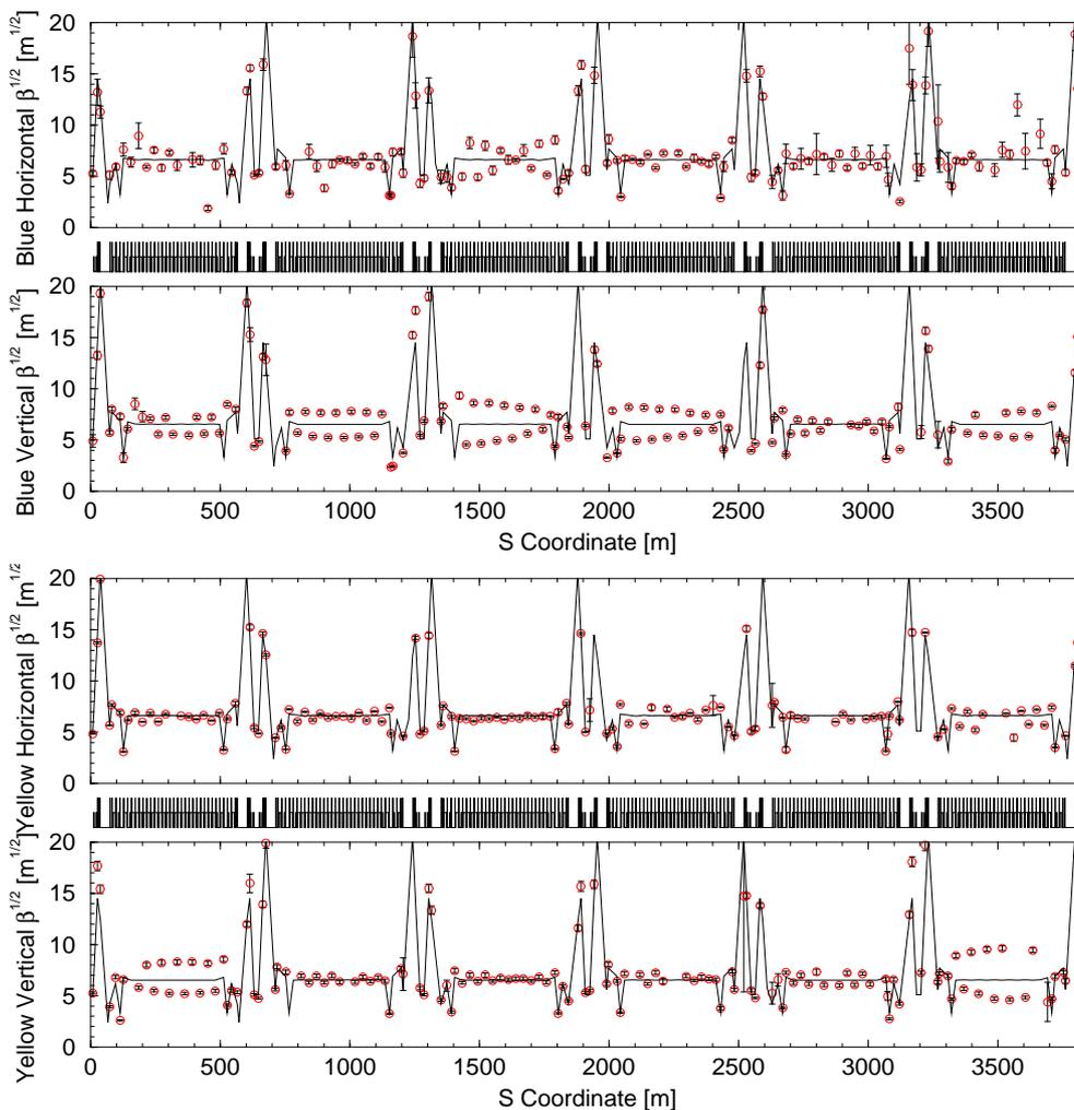
Figure 2: Measured (circles) and design (solid line) betatron functions in the RHIC Blue and Yellow rings, measured with  $\beta^*=3$  m optics at injection energy. The method of analysis is described in Section 3.1. Error bars indicate RMS variation over ten consecutive injections.
