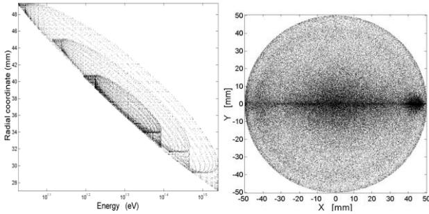
Figure 3 Energy and radial coordinate of a trapped electron
