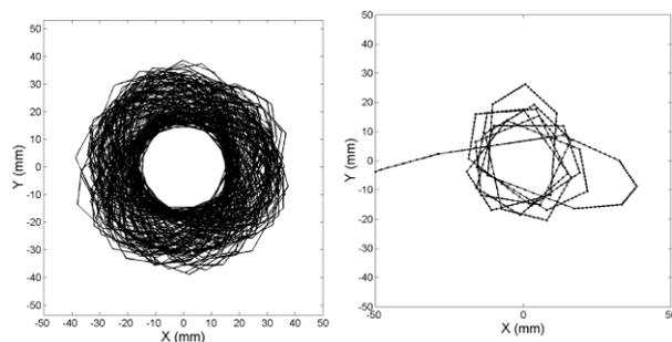
Figure 2 Orbit of tapped electron. Left: long time trapped electron; Right: short time trapped electron
