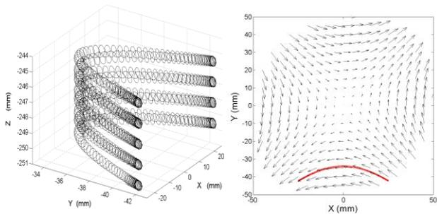
Figure 5 Photoelectron Trapping in Quadrupole Magnetic Field During the Bunch Train Gap. Left: 3D orbit; Right: 2D orbit (red line) and quadrupole field (black arrow)
