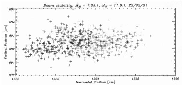
Figure 5: 1000 measurements of the spot center measured at a detector of the protein crystallography beamline.
