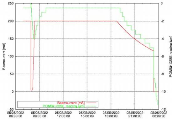
Figure 3: Movements of a BPM relative to its girder in decaying beam and top-up mode.
