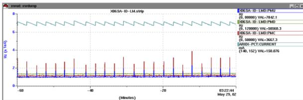
Figure 4: Particle losses during injection, measured by three loss monitors at the small gap in-vacuum undulator.
