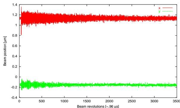
Figure 2: Measured orbit oscillations by the injection kick.
