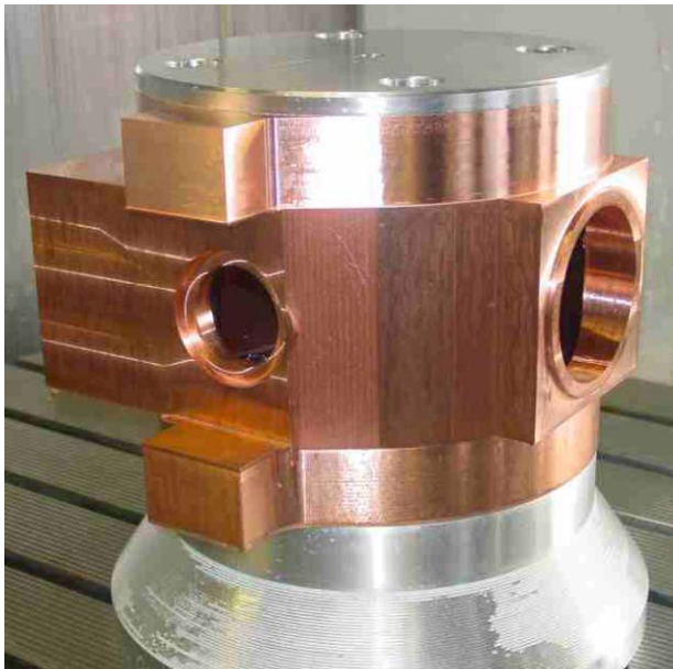
Figure 5: Bridge coupler body on mill
