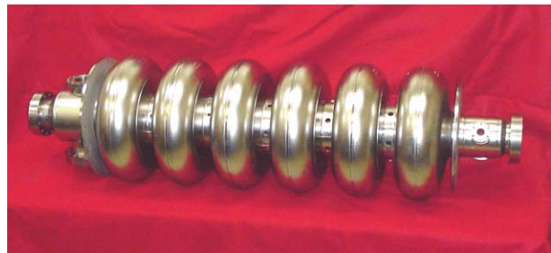
Figure 7: \beta=0.81 prototype cavity, produced by JLab courtesy Jefferson Lab
