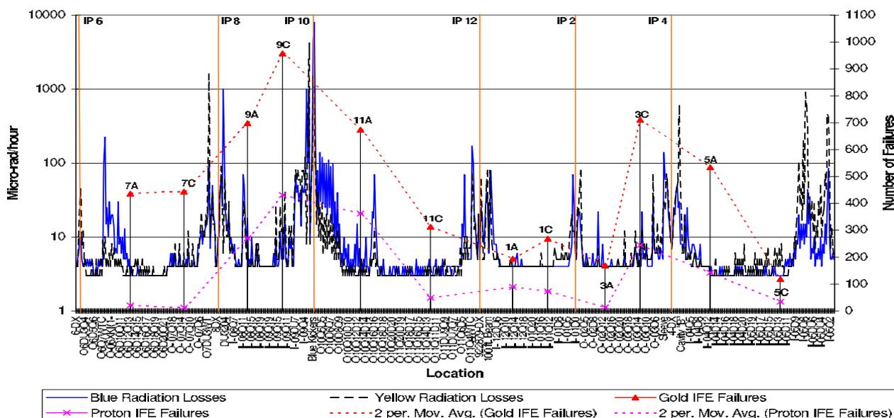
Figure 2: IFE failures and integrated beam losses in both RHIC rings for FY02–03 gold and polarized proton runs. Totals include both resettable and non-resettable failures. Labels such as 7A, 7C, etc. are RHIC tunnel alcove names where IFE signals feed into the RHIC control system. Clear correlations are visible in the region from IP8 to IP10 and around IP4. IP8 includes beam collimators; IP10 includes the beam dump.
