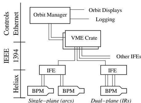
Figure 1: Architecture of the RHIC BPM system
