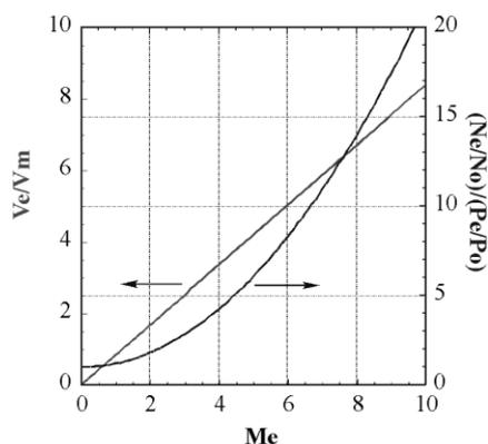
Figure 1: Figure of merit of supersonic gas injection.
