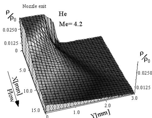
Figure 2: The density profiles of the supersonic jet near the exit of the nozzle for  $Me=4.2$  and helium obtained by the method of characteristics. Density is normalized by stagnation density at the reservoir.
