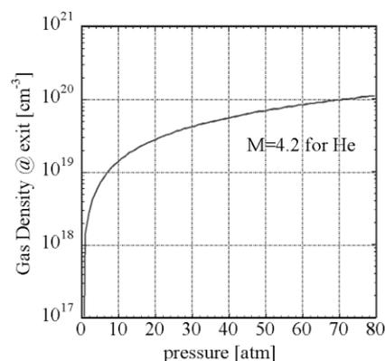
Figure 3: Gas density at the exit of the nozzle as a function of stagnation pressure at the reservoir for  $Me=4.2$  and helium.
