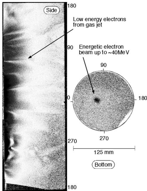
Figure 5: Typical I.P. images of electron emission at a helium gas density of  $2.1 \times 10^{19} \text{ cm}^{-3}$  and laser power of 2.9 TW.
