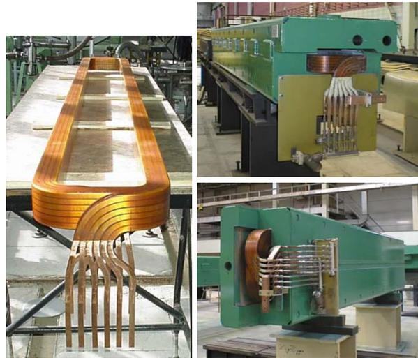
Figure 2: First MSIB coil (left), preseries magnets MSIB01 (top) and MSDC01 (bottom)
