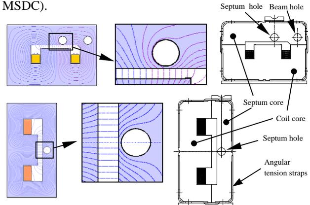
Figure 1: Field model (left) and engineering design (right) of the MSI (top) and MSD (bottom)
