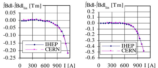
Figure 3: Nonlinearity of magnetisation curves, left: MSIB01, right: MSDC01
