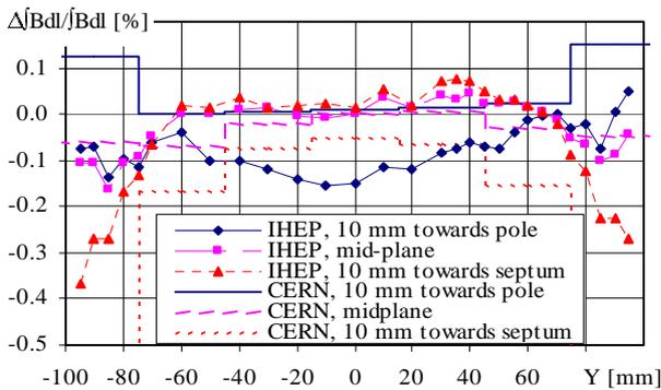
Figure 5: Transverse field homogeneity of MSDC01
