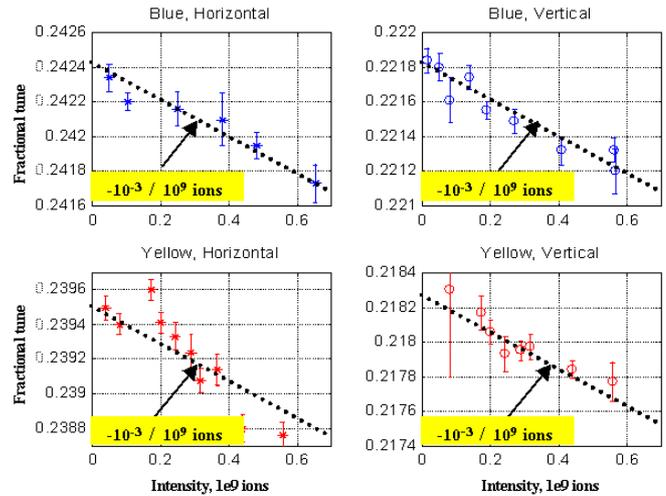
Fig.5. Tune shift vs. intensity for two rings
