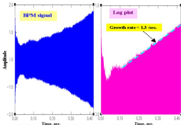
Fig.6. Resistive wall growth rate
