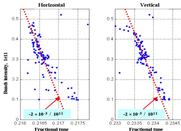
Fig.7. Tune shift measurement using PLL
