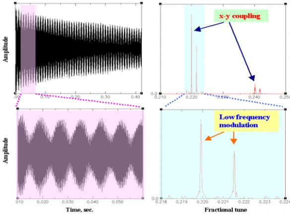
Fig.3. BPM signal and spectrum
