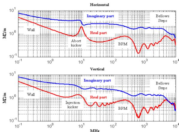
Fig.1. RHIC transverse impedance
