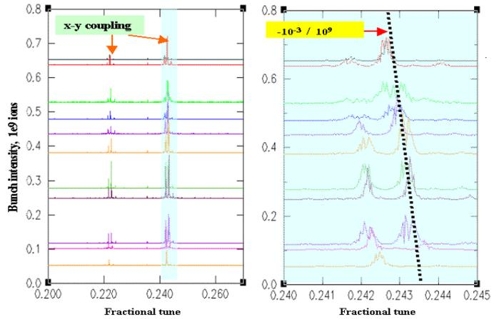
Fig.4. Mountain range of tune shift vs. bunch intensity
