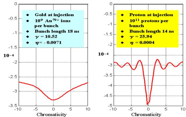
Fig.2. Expected tune shifts at injection
