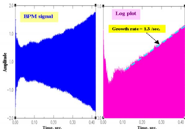
Fig.6. Resistive wall growth rate
