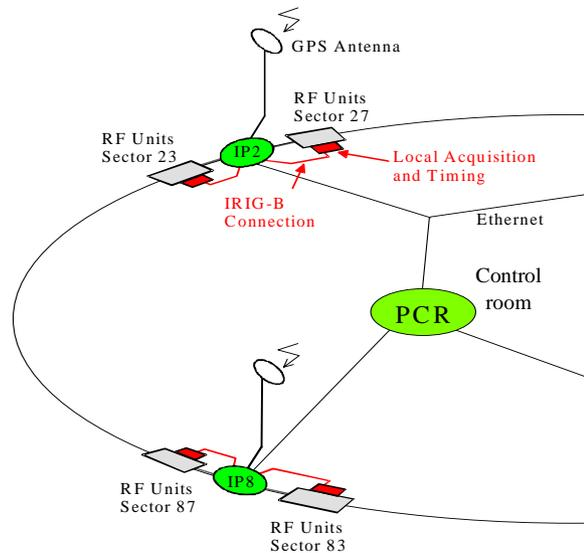
Figure 1. GPS connection to the LEP RF system
