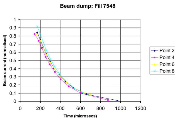
Figure 4. Beam loss measured independently in the four IPs
