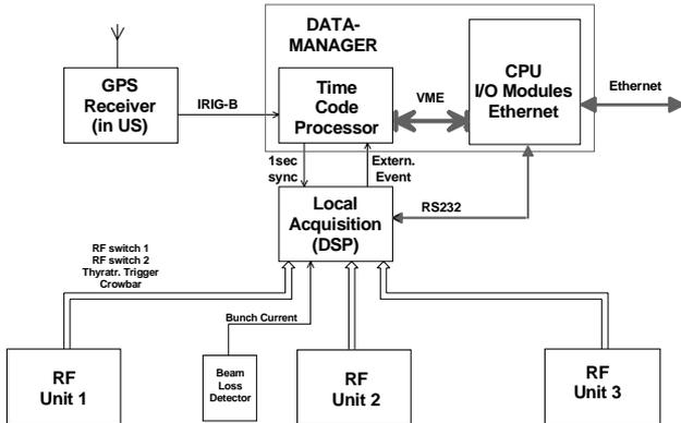
Figure 2. Local acquisition and timing in a klystron gallery
