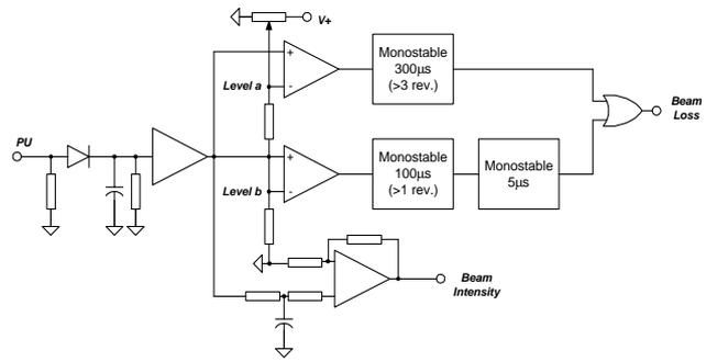
Figure 3. Beam intensity monitor and beam loss detector
