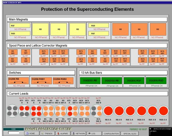
Figure 3: The main MPS panel.
