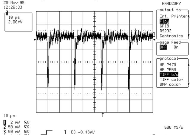
Figure 5: Structure of the current collected by the biased (+45 V) pick-up with a proton bunch density of  $7.5 \times 10^{10}$
