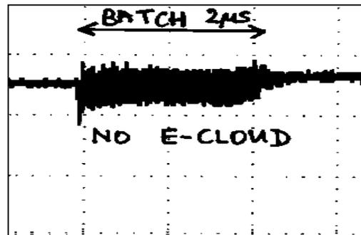
Figure 7: Vertical damper signal with a solenoid magnetic field of 100 Gauss to suppress the e'cloud ( $5.5 \times 10^{12}$  p/batch).
