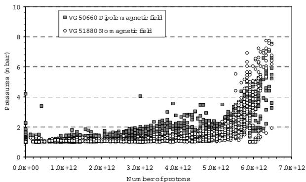
Figure 2: Pressure versus number of p/batch between two dipoles i.e. without magnetic field, duty cycle 45 %.
