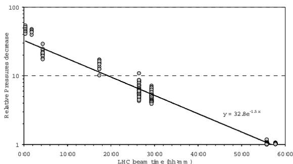
Figure 8: Relative pressure increase versus effective beam time. The effective time is the total time spent with LHC beams and bunch intensity above  $5 \times 10^{10}$ .
