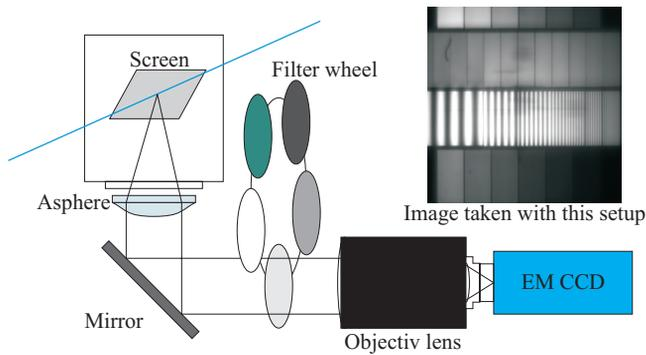
Figure 3: Layout of the imaging system for the OTR/Ce:YAG diagnostics. From the screen emitted radiation is collimated with an aspherical lens ( $f = 80$  mm) and focused by a commercial lens ( $f = 75$  mm). A motorized filter wheel allows five different attenuation factors. The small image shows a sine test pattern imaged with this setup.
