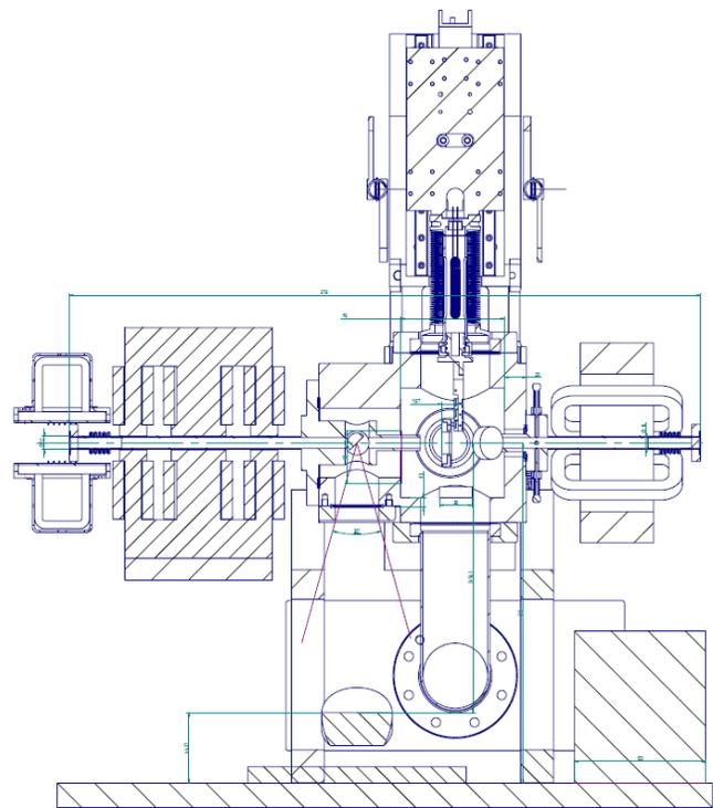
Figure 2: A sectional drawing of the sFLASH undulator intersection. Components from left to right: dipole corrector coil, phase shifter, diagnostic unit, quadrupole. The diagnostic unit accommodates a button BPM (right), wire scanners (vertical type on top), MCP for photon/electron detection and a carrier (left) with a silicon screen and a Ce:YAG crystal. The diameter of the vacuum chamber is 10 mm.
