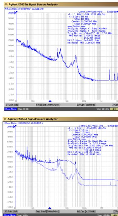
Figure 5, upper trace: phase noise of the Optical reference, 146fs<sub>RMS</sub>. Lower trace: phase noise of the remote fs laser locked to it, 461fs<sub>RMS</sub>.
