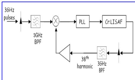
Figure 5: schematic of the remote laser synchronization to the 3GHz optical reference.
