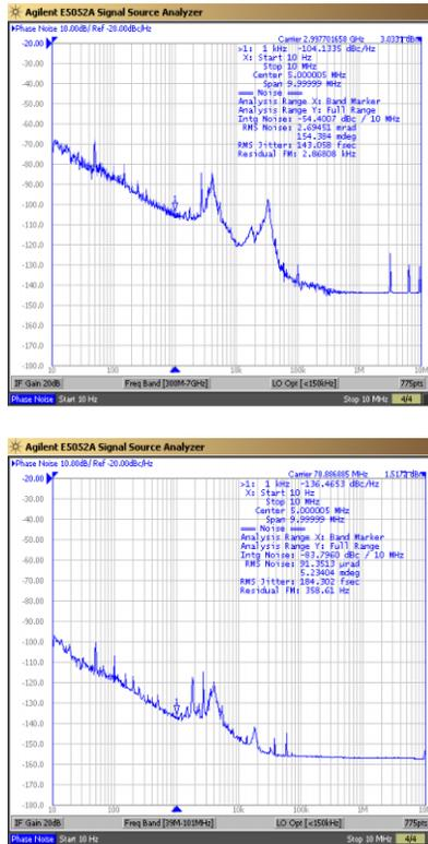
Figure 4: phase noise in the bandwidth 10Hz-10MHz of the extracted 3GHz reference, 143fs<sub>RMS</sub> (upper trace) and of the low frequency (78.86MHz) reference: 184fs<sub>RMS</sub> (lower trace).
