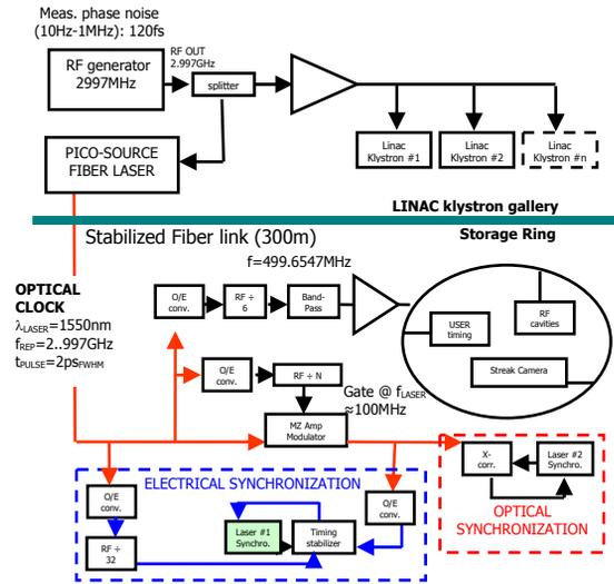
Figure 2: Optical Clock test bed at Elettra: red lines indicate optical signals, blu lines indicate electrical signals.
