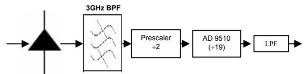
Figure 3: block diagram of the "direct conversion".
