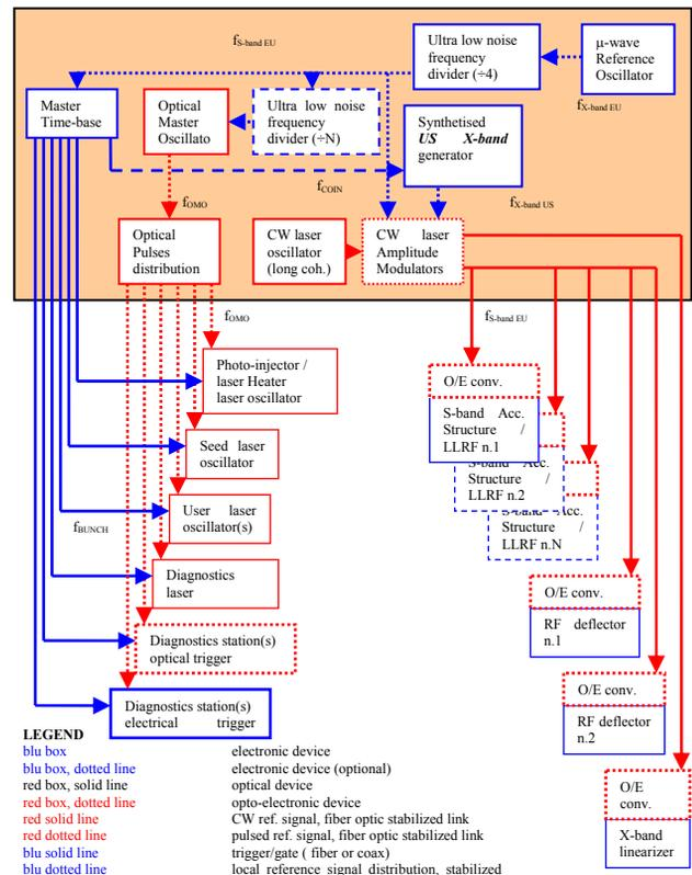
Figure 1: Block diagram of the FERMI timing system.
