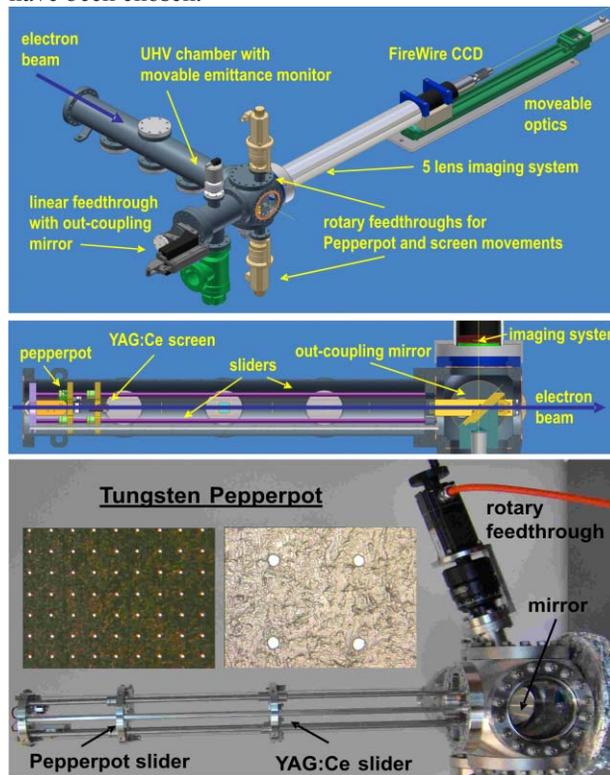
Figure 3: Schematic drawing of emittance monitor and imaging system (top), cross section of UHV part showing the sliders for the “pepperpot” and scintillation screen (middle), photograph of the emittance monitor (without UHV chamber) and “pepperpot mask” (bottom)
