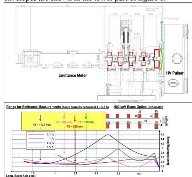
Figure 1: Mechanical drawing of 1<sup>st</sup> phase of LEG test facility (upper part). Optics simulations for expected beam current range showing beam envelopes at locations of smallest transverse emittances (lower part). The measuring range of the emittance monitor is indicated in yellow.
