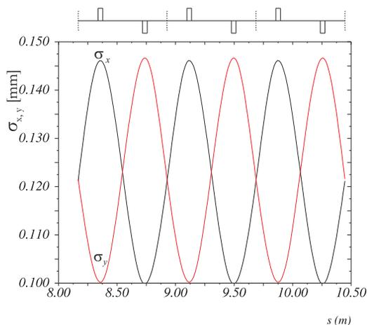
Figure 2: RMS beam size inside the FODO lattice for a beam with zero current. The abscissa coordinates are shifted with respect to the entrance of the matching section so that  $s = 0$  corresponds to the beginning of the drift space in front of the first matching quadrupole.
