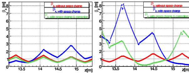
Figure 4:  $\beta_x$  (left) and  $\beta_y$  (right) along the tomography section. Inverting the quadrupoles' gradients along the tomography and matching sections delivers the same periodic solution for  $\beta_y$ .
