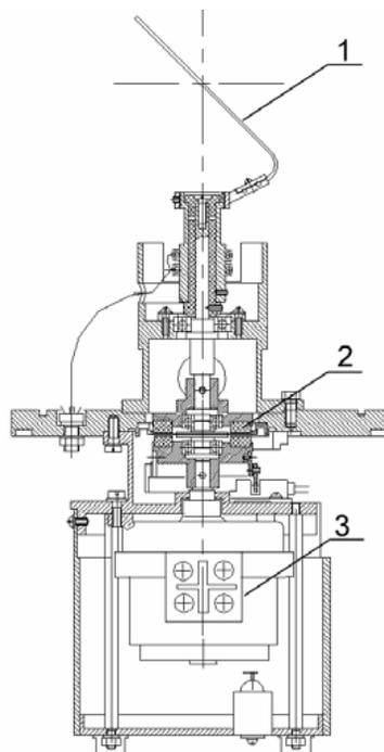
Figure 3: The sketch of the rotating wire scanner, where:
