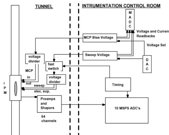
Figure 2: Block diagram of the IPM system
