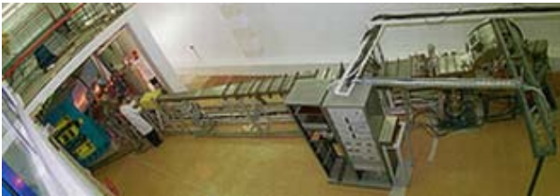
Figure 5: Extracted beam transportation line. From left side is cyclotron, from right side is irradiation installation
