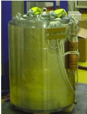
Figure 6:SECRAL superconducting magnet assembly.
