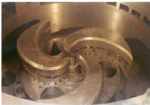
Figure 3: Pole tips installed on the pole base.
