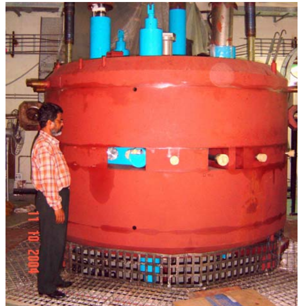
Fig.2: Cyclotron magnet with cryostat installed in it.
