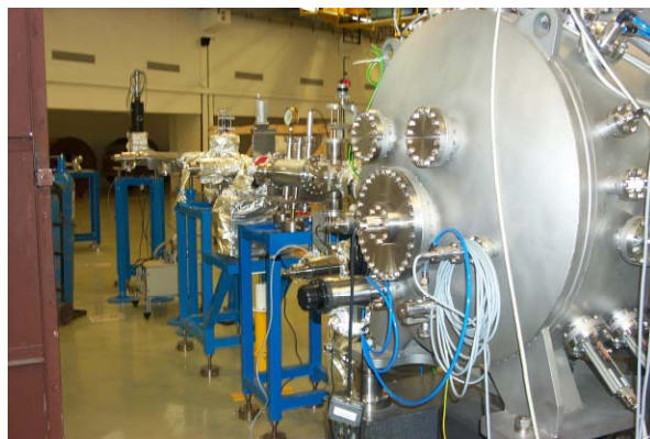
Figure 10: Down stream view of the XRD beamline. The large chamber in picture houses the DCM.
