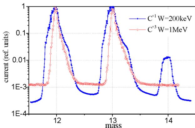
Figure 4: Mass spectrums of accelerated beams. The molecules of 14 mass are destroyed in stripper.
