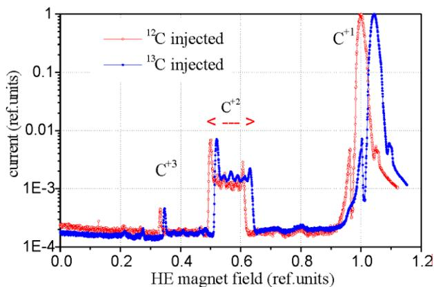
Figure 5: The scans of the HE magnet with  $^{12}\text{C}$  and  $^{13}\text{C}$  ions
