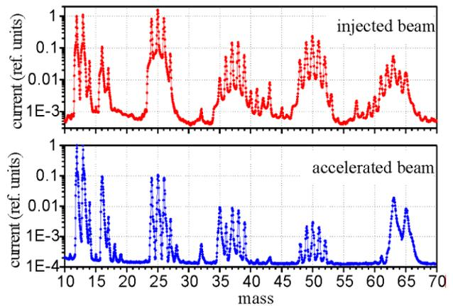
Figure 1: Mass spectrums of the <sup>13</sup>C enriched graphite with (<sup>12</sup>C)<sub>m</sub>(<sup>13</sup>C)<sub>n</sub> clusters
