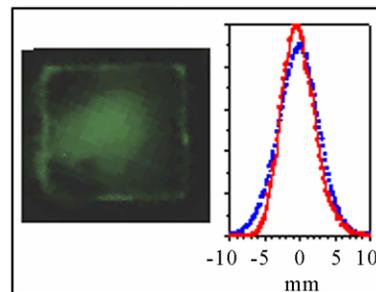
Figure 3: Beam photo from “CsI” crystal and profile at the exit of the AMS.
