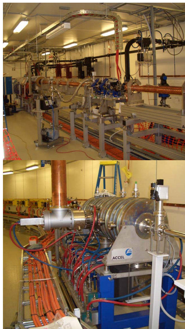
Figure 4: Normal conducting 3 GHz linac (top) and 500 MHz booster cavity (bottom) installed at the Australian Synchrotron project.
