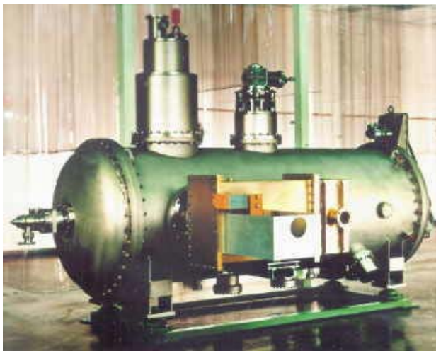
Figure 1: Superconducting accelerator module housing one 5-cell 500 MHz module completely assembled and tested prior shipment to JAERI site.
