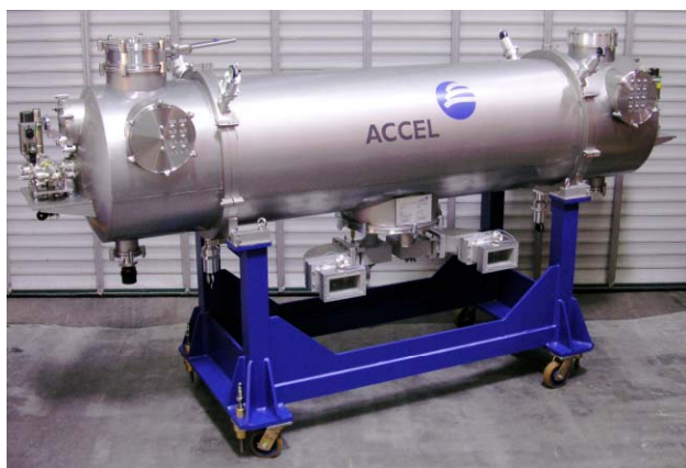
Figure 3: Superconducting Rossendorf style 1.3 GHz module prior shipment to Daresbury. Peking University is planning to use this module for their FEL application.
