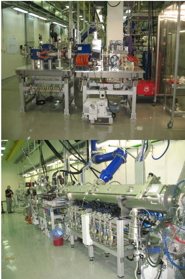
Figure 5: ECR ion source (top) and RFQ (bottom) installed at the SARAF accelerator of the SOREQ institute in Israel
