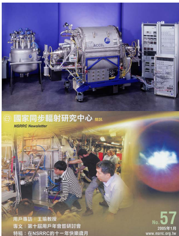
Figure 2: Completely assembled and tested first superconducting 500 MHz module with valve box and SRF electronics ready for shipment to NSRRC (above) and during installation into the NSRRC storage ring (bottom)
