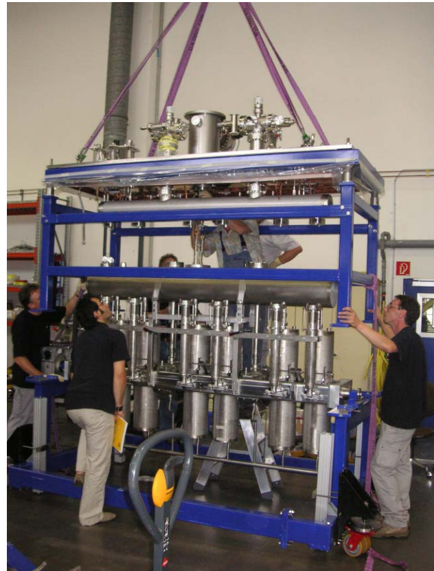
Figure 6: Assembly of the superconducting 176 MHz accelerator module for proton/deuteron acceleration. The module houses 6 halfwave resonators and 3 superconducting solenoids
