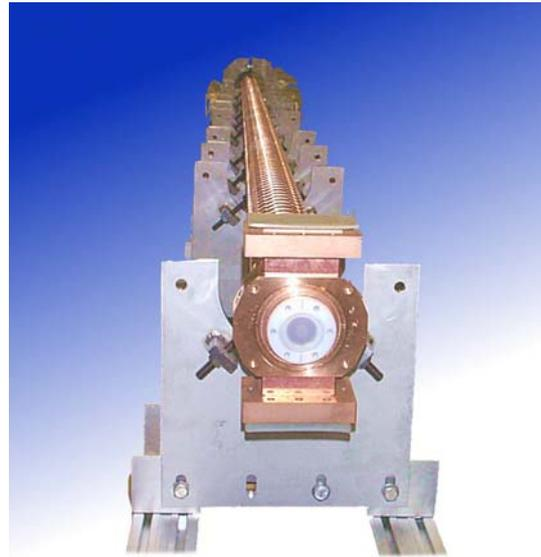
Figure 5: 5.2m long 3 GHz S-Band accelerating structure
