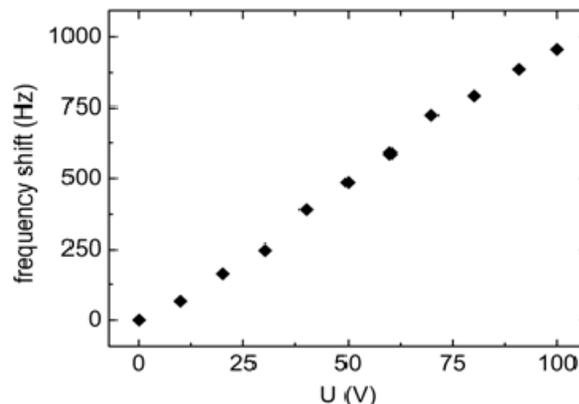
Figure 2: Measurement of the resonant frequency of a S-DALINAC cavity using a piezo tuner at 2 K. The plot shows the shift of the resonance frequency as function of the piezo voltage.
