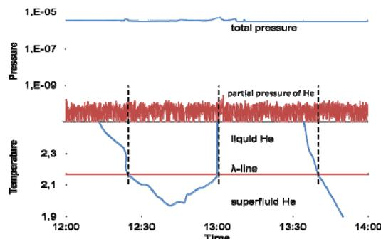
Figure 3: Temperature cycles through the lambda-point of liquid helium did not increase the leak rate.
