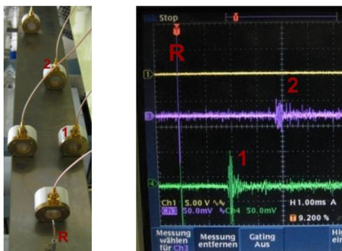
Figure 5: In house developed and built OSTs in a test set-up and oszilloscope screenshot of successful test. R labels the electrically pulsed resistor exciting the second sound wave and 1 and 2 the corresponding OSTs and their electrical response signals.
