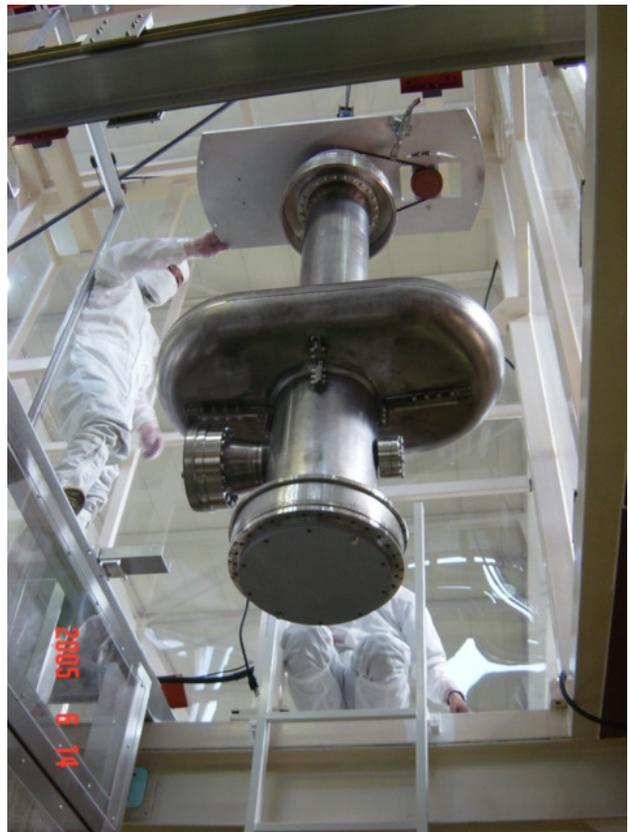
Figure 7: High pressure rinsing; KEKB crab cavity #2 with transition flange under high pressure rinsing.
