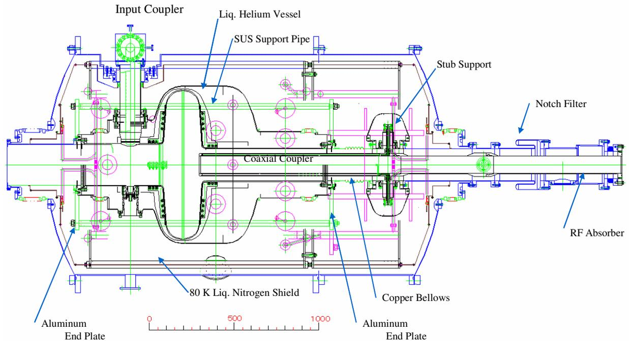
Figure 10: Detailed design of the KEKB crab cavity (Top view).
