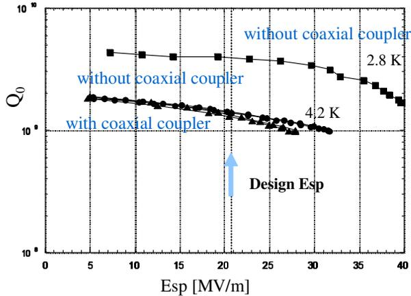
Figure 5: Measured  $Q_0$  of KEKB crab cavity #1 without and with coaxial coupler.
