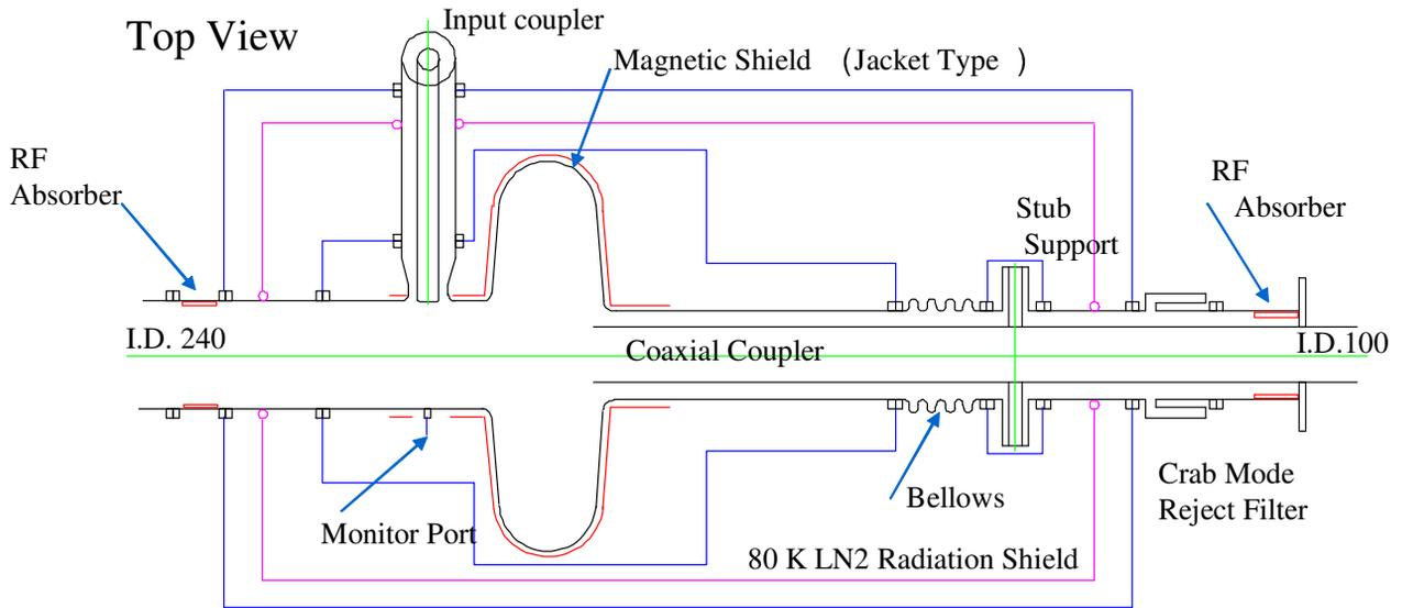
Figure 8: Conceptual design of the KEKB crab cavity in the horizontal cryostat.
