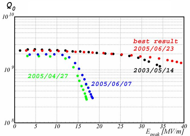
Figure 6: Measured  $Q_0$  of KEKB crab cavity #2.
