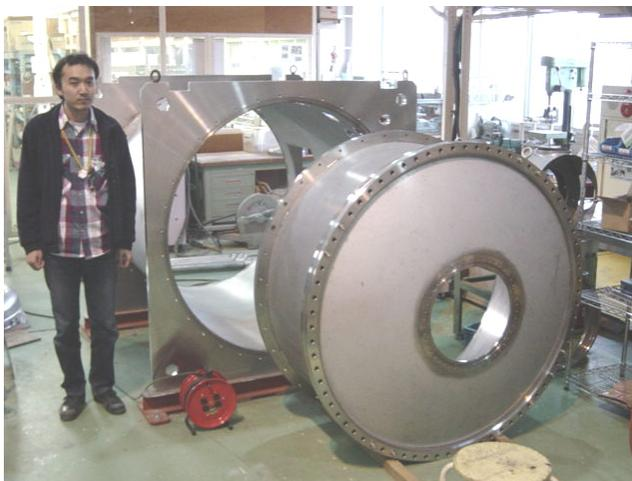
Figure 13: Vacuum vessel for KEKB crab cavity.
