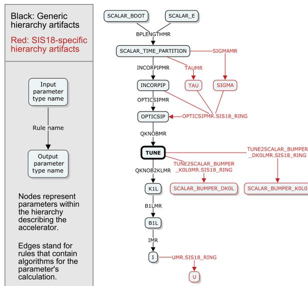
Figure 2: Hierarchy for inputs and outputs of the tune parameter type, showing how distinctive features of SIS18 are added while keeping the generic ring accelerator model structure intact.
