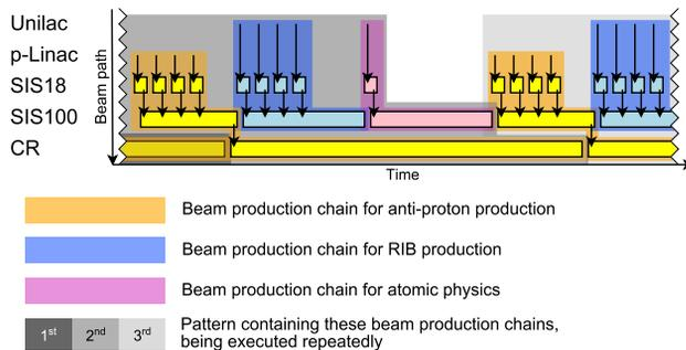
Figure 3: Example for parallel beam operation showing aggregation of beam process chains into patterns. HESR accumulating the anti-protons is omitted.
