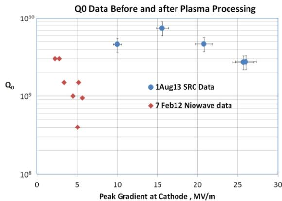
Figure 2: Calorimetric  $Q_0$  data for cavity.
