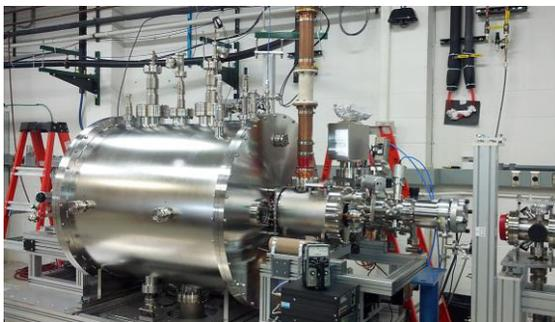
Figure 1: Electron gun installed in vault.
