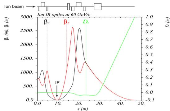
Figure 1: Detector region optics in the MEIC ion collider ring.
