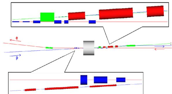
Figure 3: Layout of magnets in the detector region of MEIC collider rings.
