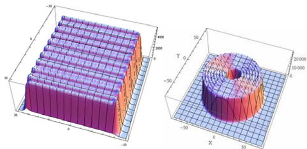
Figure 4: An example of generic square raster-scanned beam (left), and generic circular scanned beam (right) that D-Pace's standard product AC Scan Magnets can deliver. The customer shall tailor the undisclosed beam distributions on target according to their own proprietary algorithms through D-Pace's programmable two channel signal generator.
