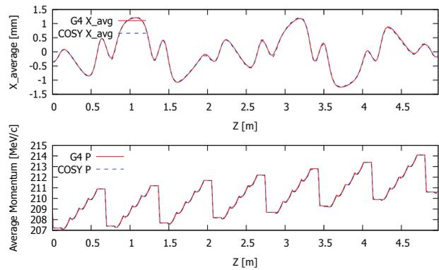
Figure 2: Average Momentum and X as a function of Z for the beam in G4beamline and COSY.
