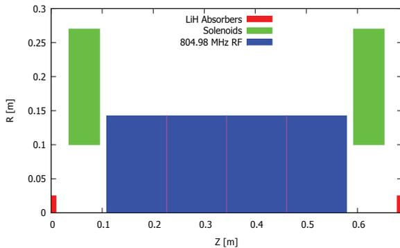
Figure 1: R vs. Z geometry of 1 cell.
