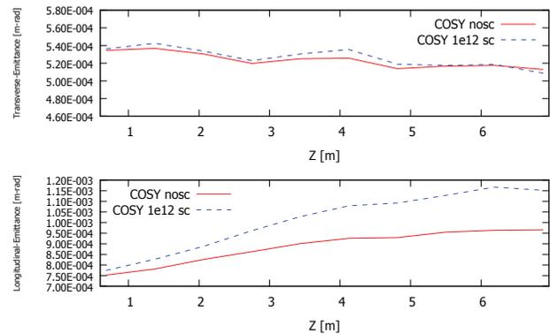
Figure 3: Transverse and Longitudinal beam emittance over 10 cells in COSY with and without space charge.
