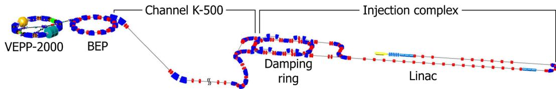
Figure 9: Layout of the facilities related to the VEPP-2000 collider after upgrade.
