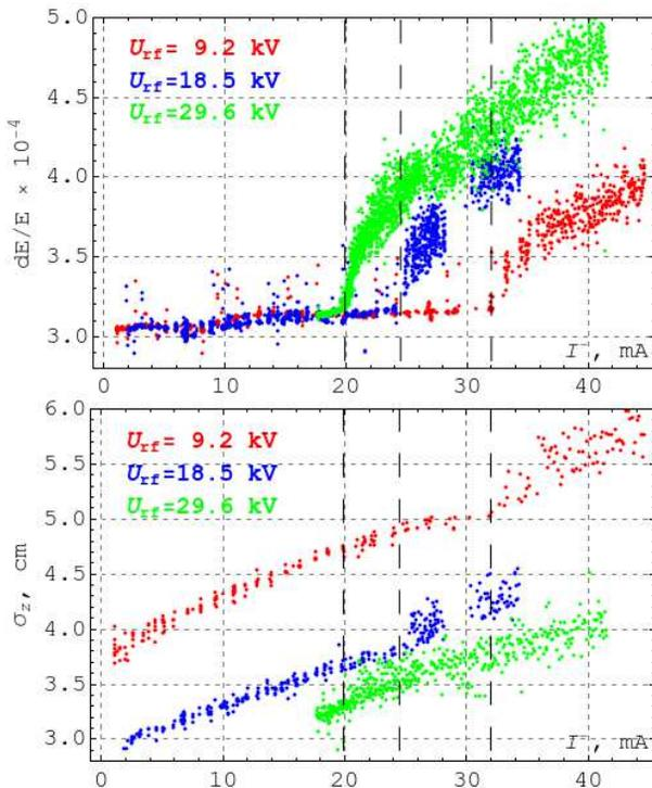
Figure 7: Correlation of the current dependence of the extracted energy spread and the measured bunch length.
