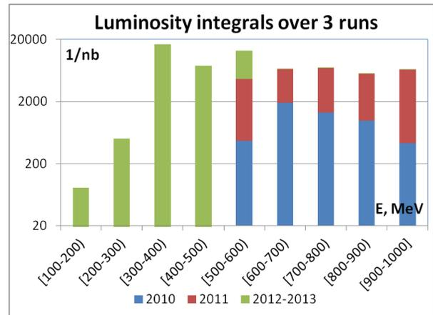
Figure 5: Luminosity integrals collected by SND in different energy ranges over the entire VEPP-2000 operation time.
