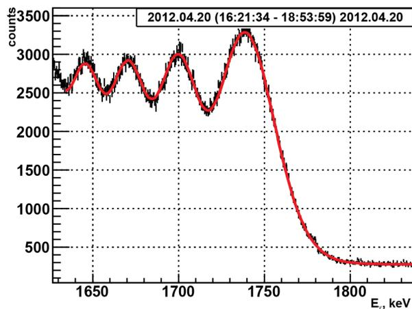
Figure 2: Compton backscattering spectrum at VEPP-2000. Reconstructed energy is  $E = 993.662 \pm 0.016 \text{ MeV}$ .
