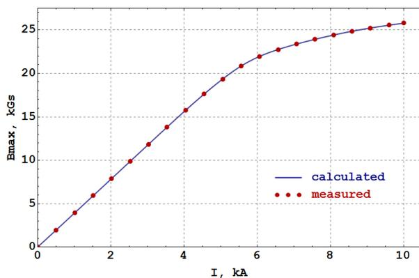
Figure 10: Comparison of the calculated and measured magnetic field vs current for the upgraded BEP dipole.
