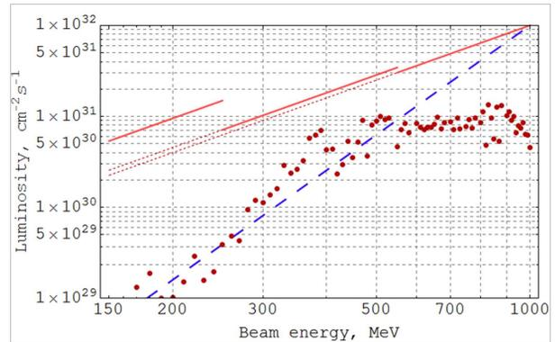
Figure 4: Luminosity dependence on energy. Lines – the theoretical estimations; dots – performance in best runs over the entire VEPP-2000 operation time.
