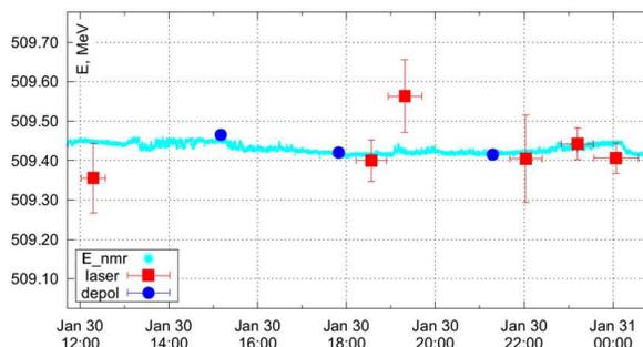
Figure 3: Comparison of three different methods of energy measurements: blue circles – resonance depolarization; red squares Compton backscattering; light-blue curve – calibrated NMR.
