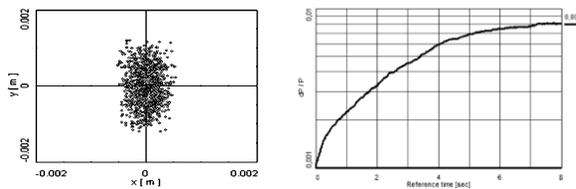
Figure 5: Antiproton beam interaction with the Helium target. E=30 keV. Left: Beam spot at target location; Right: evolution of rms momentum spread of 30 keV antiprotons.
