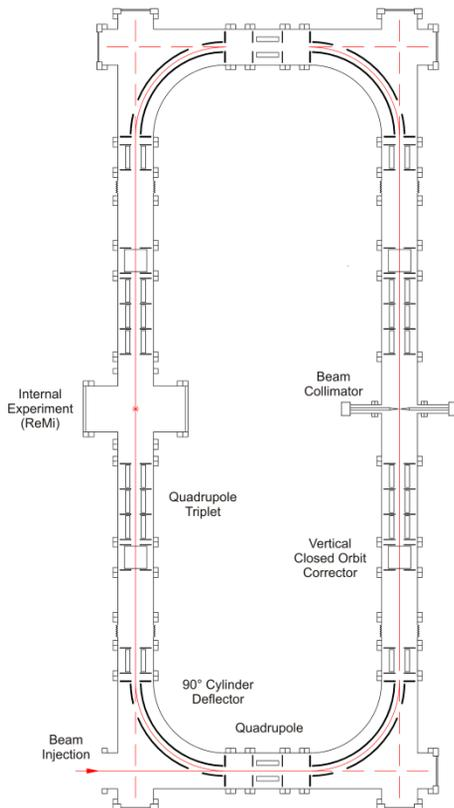
Figure 1: Scale layout drawing of the recycling ring.
