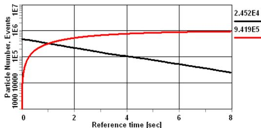
Figure 4: Beam intensity losses and integral of ionization events at E=30 keV (life time ~4s).
