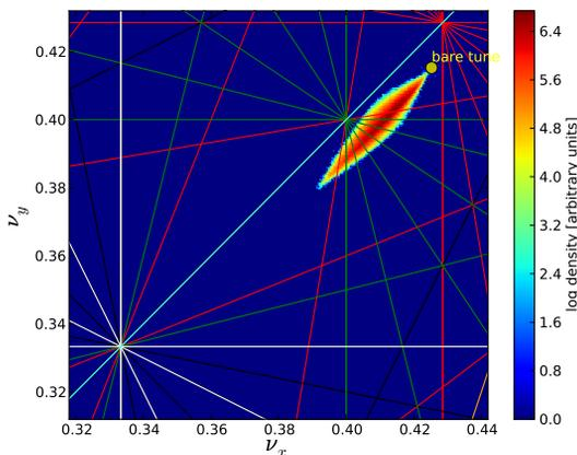
Figure 4: The tune footprint spread out by space charge at the current nominal settings.
