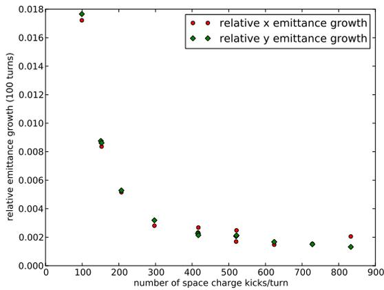
Figure 3: The relative space charge induced emittance growth  $(\epsilon_f - \epsilon_i)/\epsilon_i$  over a 100 turn simulation varying the number of space charge kicks per turn.
