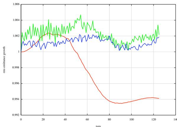
Figure 1: The RMS emittance growth as a function of turn number for a zero current, ML/I-generated bunch matched using a third order normal form. The horizontal, vertical, and longitudinal emittances are shown in green, blue, and red, respectively.
