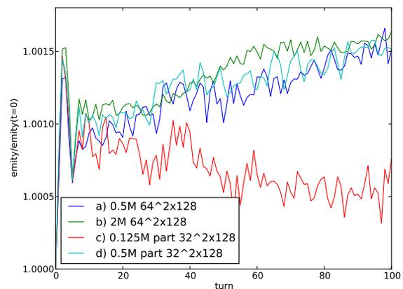
Figure 2: The emittance calculated over a 100 turn run for different numbers of macroparticles and grid size: a) 0.5 million,  $64 \times 64 \times 128$ ; b) 2 million,  $64 \times 64 \times 128$ ; c) 0.125 million,  $32 \times 32 \times 128$ ; d) 0.5 million  $32 \times 32 \times 128$ .
