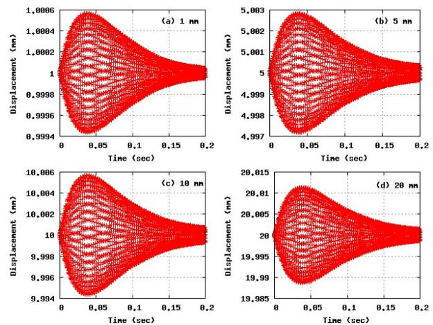
Figure 4: Transverse displacement versus time for different beam initial offsets monitored at the exit of final beamline element.  $Q = 5 \times 10^{10}$  and initial current = 1 mA.
