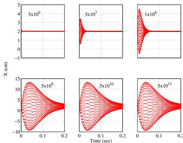
Figure 2: Transverse displacement versus time monitored at the exit of the final beamline element. Subplots correspond to different  $Q$ -values as shown. The beam has initial offset of 20 mm and 100 mA current.
