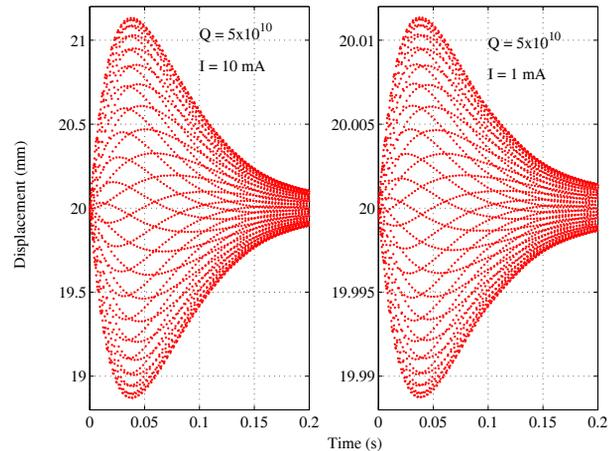
Figure 3: Transverse displacement versus time for 1 mA and 10 mA beam current with  $Q = 5 \times 10^{10}$  and 20 mm initial beam offset at the exit of final beamline element.
