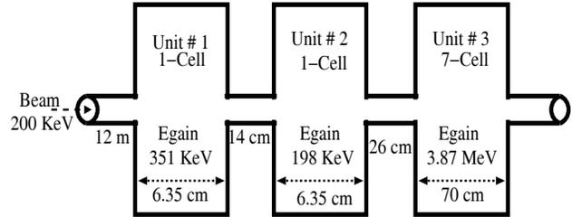
Figure 1: Schematic layout of the system considered in the simulations.
