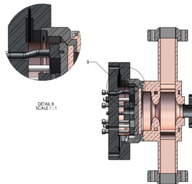
Figure 4: Cathode system mechanical drawing.
