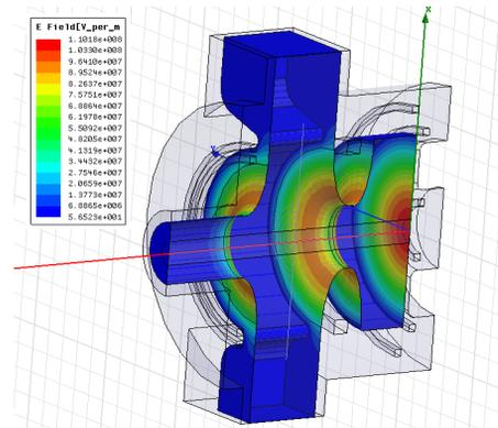
Figure 1: 3D model used for HFSS simulation. Surface electric field is shown.
