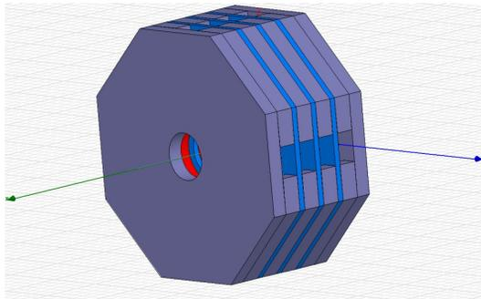
Figure 5: Solenoid for emittance compensation.
