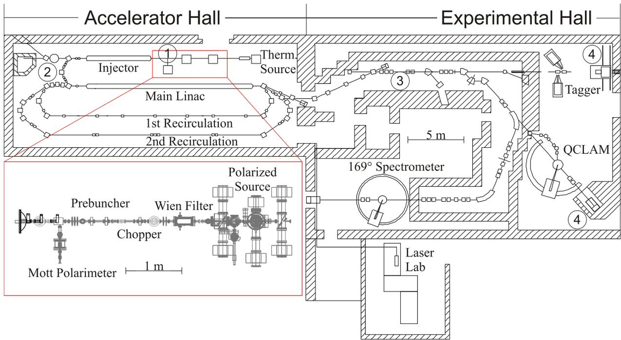
Figure 1: Layout of the S-DALINAC. The polarized source seen in the inset on the lower left is installed between the thermionic source and the superconducting injector linac. The laser beam is transported through an optical fiber (diode laser) or an evacuated laser beam transport line (Ti:Sapphire laser). The positions of the various polarimeters are as follows: 1. 100 keV Mott polarimeter; 2. 5-10 MeV Mott polarimeter; 3. 50-130 MeV Møller polarimeter; 4. Compton transmission polarimeters
