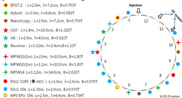
Figure 3: Layout of PLS-II storage ring ID distribution
