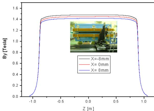
Figure 2: Central field profile of combined function bending magnet for the PLS-II
