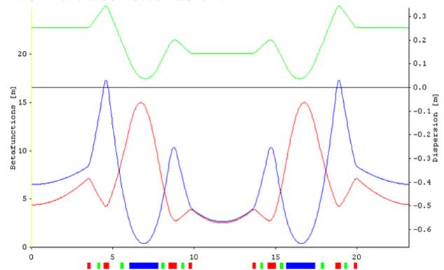
Figure 1: Magnetic lattice and Twiss functions for one cell of the PLS-II
