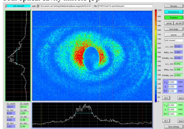
Figure 1: Retro-reflected HeNe used in alignment procedure.
