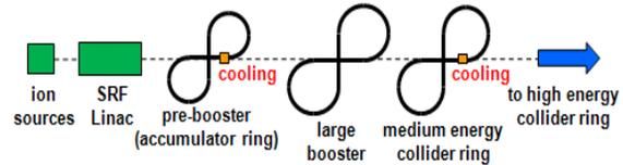
Figure 3. A schematic layout of MEIC ion complex.
