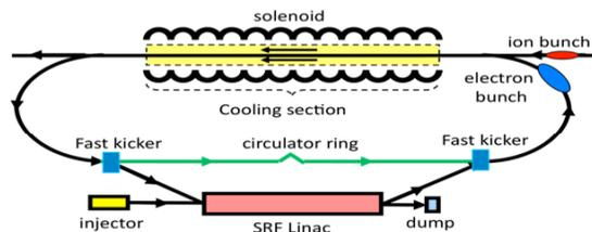
Figure 5: Schematic of electron cooling for the MEIC.
