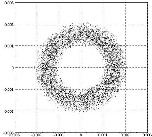
Figure 3: Cross-section of the real particle distribution in the beam on the target. Axes dimensions are given in meters.
