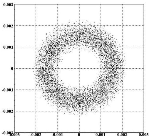
Figure 5. Cross-section of the real particle distribution in the beam with beam's current on the target. Axes dimensions are given in meters.
