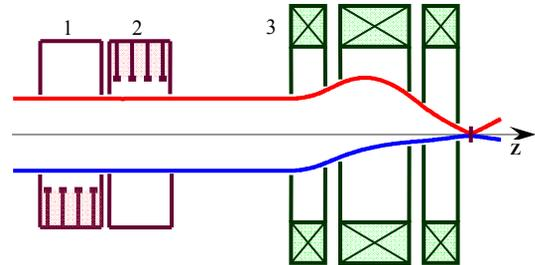
Figure 1: Preliminary designed layout of the system for hollow beam formation. Where 1 – horizontal deflector; 2 – vertical deflector; 3 – focusing system.
