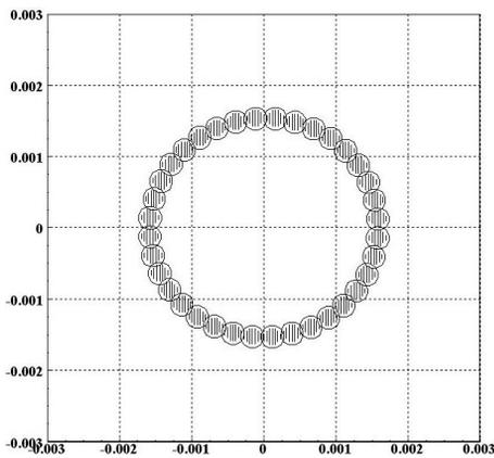
Figure 2: Cross-section of the monochromatic beam on the target. Axes dimensions are given in meters.
