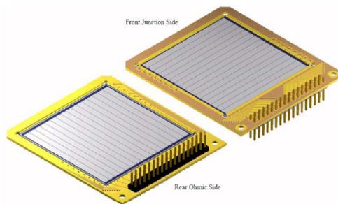
Figure 4: The two sides of a Double Sided Silicon Strip Detector (DSSSD).
