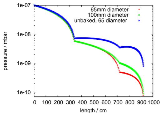
Figure 4: Pressure along the new beamline.
