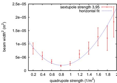
Figure 7: Quadrupole scan.
