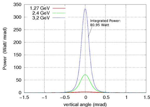
Figure 3: Power of the synchrotron light at ELSA depending on the vertical angle.
