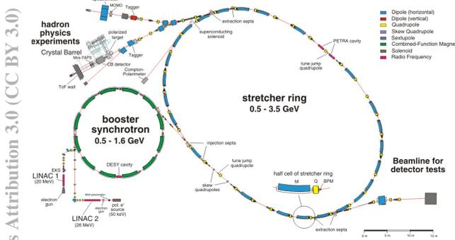
Figure 1: Electron Stretcher Facility ELSA.
