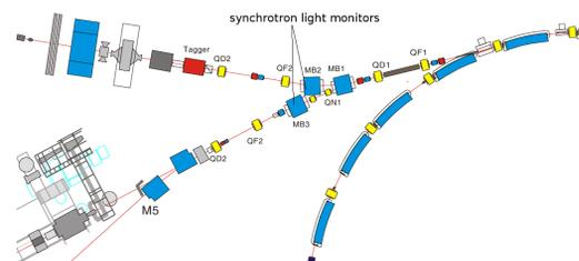
Figure 5: Synchrotron light monitors at the external beamline.
