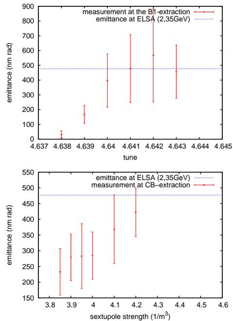
Figure 8: Emittance depending on the extraction parameters. The blue line shows the equilibrium emittance at the stretcher ring.
