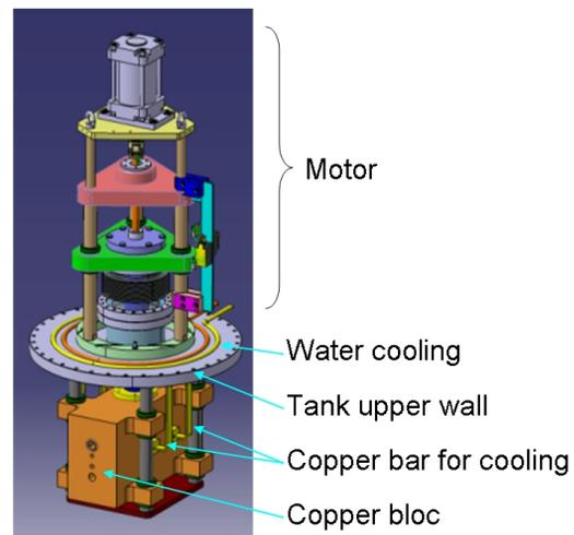
Figure 4: Collimator design.
