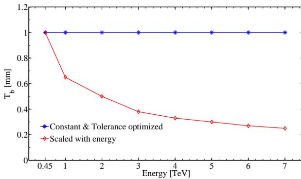
Figure 1: Tolerance budget  $T_b$  as a function of beam energy for different collimator settings.
