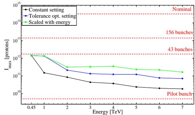
Figure 2: Maximum beam intensity reach for a minimal one-stage cleaning system. A 0.1 h beam lifetime is considered.
