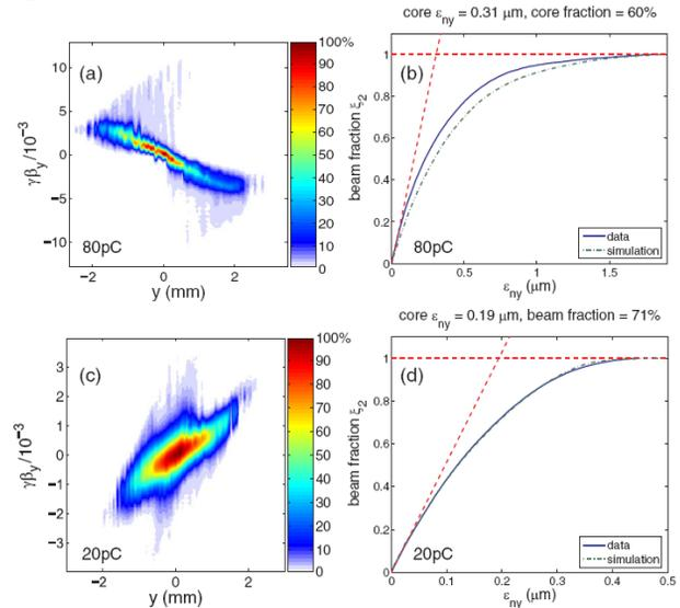
Figure 5: Measured (a), (c) transverse phase space after the gun and the corresponding emittance versus beam fraction curve (b), (d).
